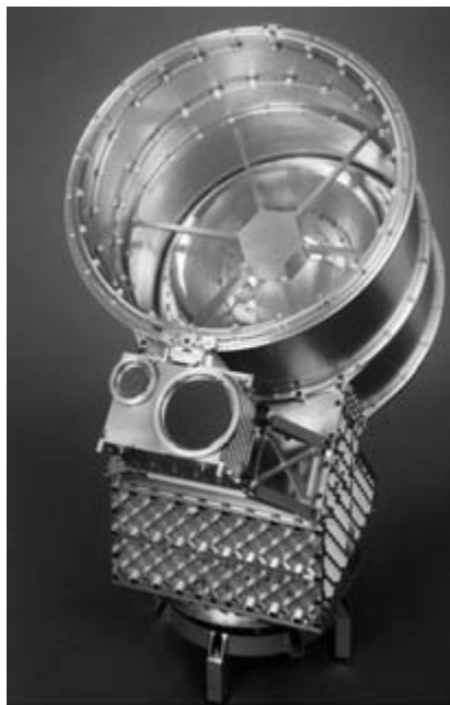
Figure 3. Cosmic Dust Analyzer on Cassini. The detector has a sensitive area of 0.1 \text{ m}^2 and is based on the impact ionization effect: A dust particle which enters the detector and hit the gold target at speed above 1 \text{ km/s} will produce an impact crater and free electrons and ions are generated. These ions and electrons are separated in an electric field within the detector and collected by electrodes. The strength and the wave form of the signal are measures of the mass and speed of the impacting particle. A combination of an impact ionization detector with a mass spectrometer gives the chemical composition of the produced ions.
